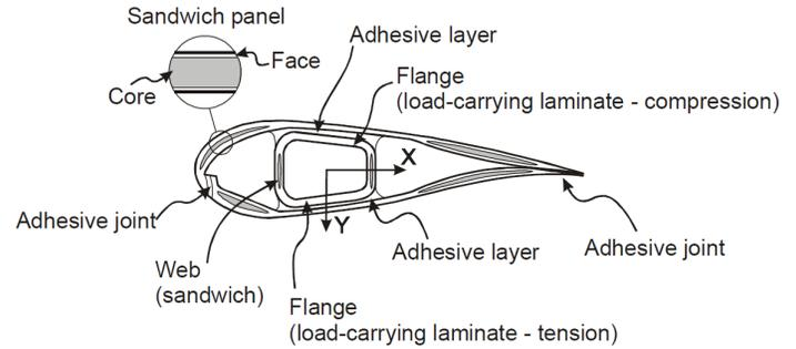
**FIGURE 4.** Nomenclature and used materials in a conventional blade structure [3].
