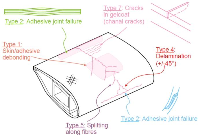
**FIGURE 2.** Sketch of common damage types found on a wind turbine blade [3].
