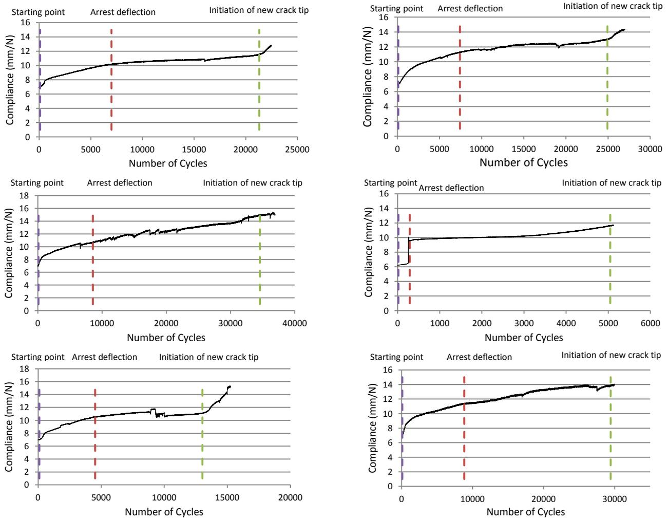
Fig. 5. Compliance – Number of cycles relation for the six beams loaded in fatigue. The borders reflect three different stages of life cycle of the beams. a) Starting point, initiation of the fatigue life cycle after crack has reached the lower interface, b) Arrest deflection, the maximum deflection length of the crack inside the peel stopper, c) Initiation of new crack tip, the time where a new crack face is created at the other side of the peel stopper
