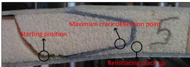
Fig. 6. The three stages of crack evolution in the sandwich beam
