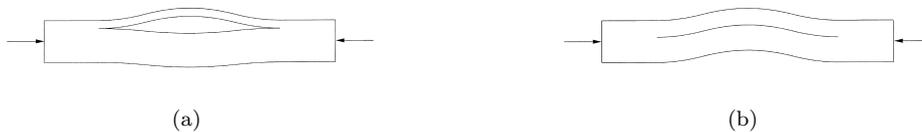
**Figure 2.9:** (a) Local and (b) global buckling mode visualised for plates exposed to compressive loading (taken from Short et al. [109]).
