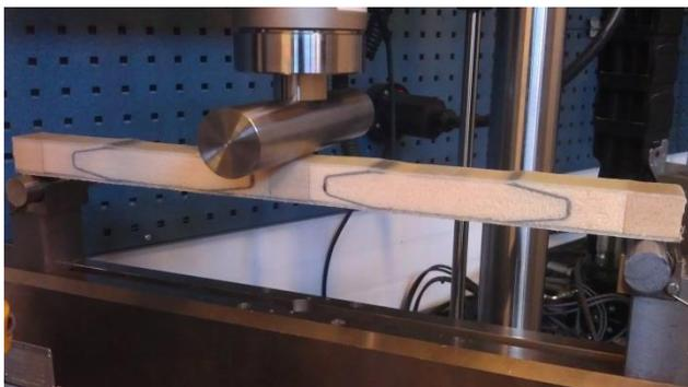
Fig. 1. Sandwich beam specimen in 3-point bending testing rig.
