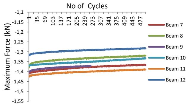
Fig. 4. Force at maximum displacement for the last 500 cycles of the crack initiation routine.
