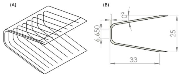
Fig. 2. (A) Fiber reinforced peel stopper design and fiber alignment. (B) Cross section of the peel stopper sheet.
