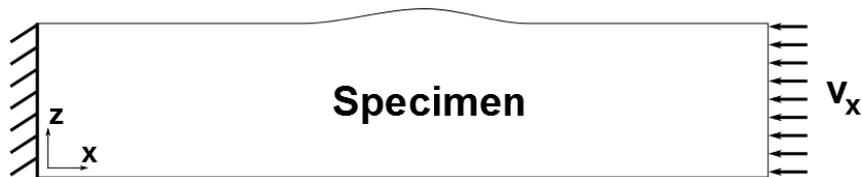
Figure 2: Boundary conditions for the model.
