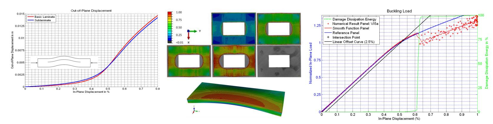
Figure 5: Global buckling in small scale panel simulation
