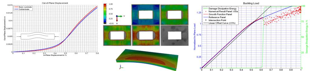
Figure 5: Global buckling in small scale panel simulation
