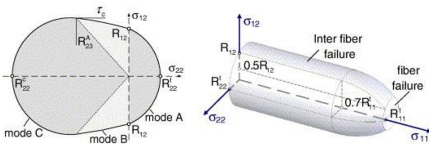
Figure 2: Puck failure criterion envelop
