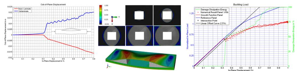
Figure 4: Local buckling in small scale panel simulation
