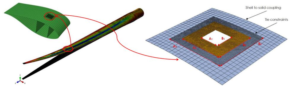
Figure 3: Large scale delamination simulation with cohesive elements
