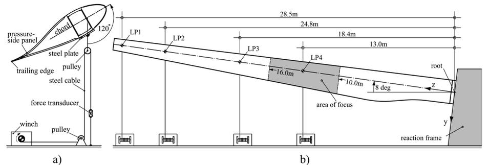
Figure 4: a) Cross section with pulley system and force transducer, b) Elevation of test setup with LP positions and area of measurement focus.
