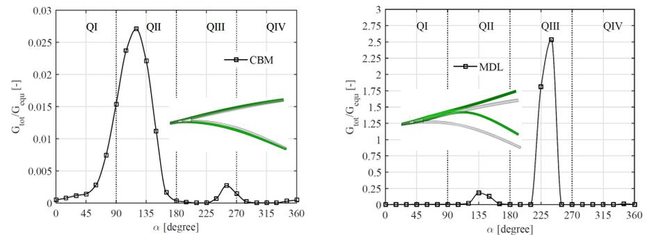
Figure 5:  $G_{tot}/G_{equ}$  as a function of the bending moment vector angle  $\alpha$  and its magnitude subdivided into four quadrants indicated by dotted lines for a constant bending moment (CBM) and the maximum design load (MDL).
