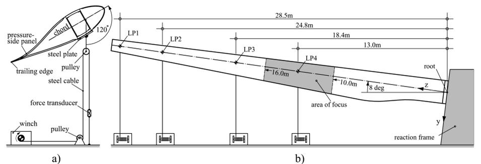
Figure 4: a) Cross section with pulley system and force transducer, b) Elevation of test setup with LP positions and area of measurement focus.
