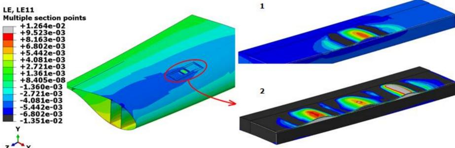
Figure 3: Local cap opening buckling mode with stable crack growth ( $t/T=7.5\%$ ,  $b/B=0.40$ ).
