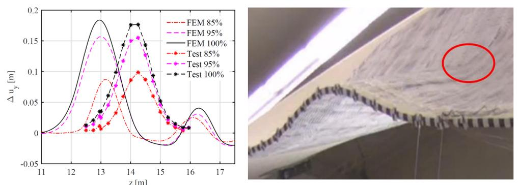
Figure 6: Comparison of local deformation as offset from a curve fit through the global displacement. Trailing edge deformation just before reaching the ultimate load. Note the distinct kink at the upper surface.
