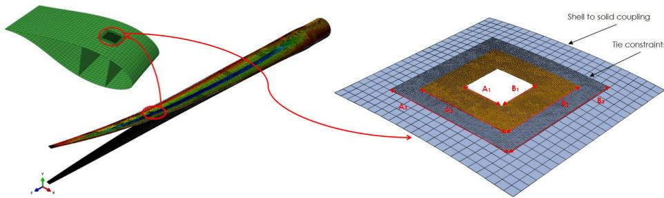
Figure 2: Large scale delamination simulation with cohesive elements
