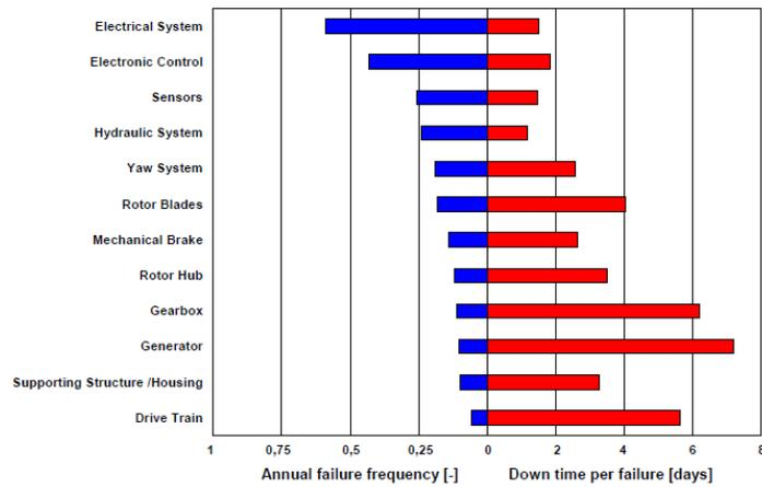
FIGURE 1. Failure Frequency and downtimes of components [1].
