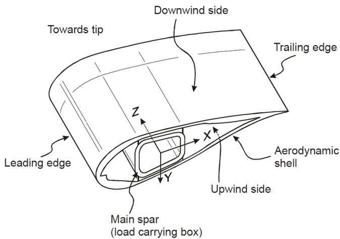
**FIGURE 3.** Main components of a rotor blade [3].
