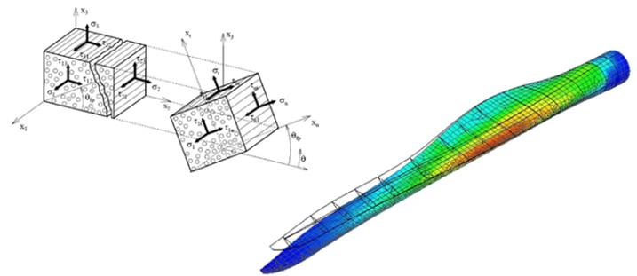
**FIGURE 5.** Qualitative illustration of multi axial stress states in a wind turbine rotor blade.
