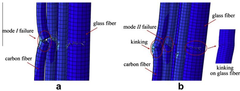
Fig. 15. Different failure modes under tension loading period (a) and compression loading period (b).
