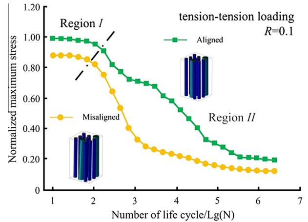
Fig. 8. S–N curves of hybrid composites with aligned and unaligned fibers.
