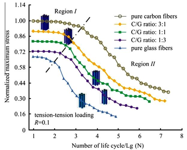
Fig. 2. Comparison of the  $S$ – $N$  curves of HFRC with different carbon/glass ratios.
