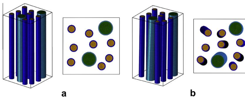
Fig. 7. FEM unit cell models of (a) aligned and (b) misaligned hybrid composites, general and top views.
