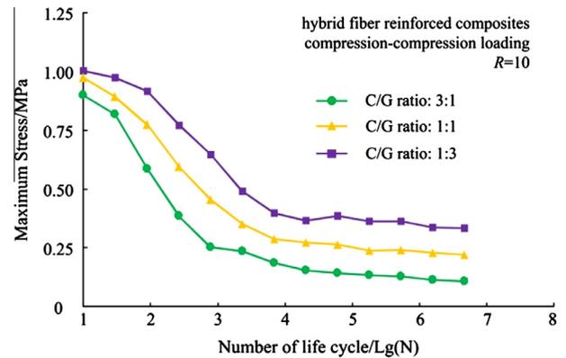
Fig. 11. S–N Curves of different hybrid composites under compression–compression cyclic loading. Vertical axis is normalized by 314.54 MPa.
