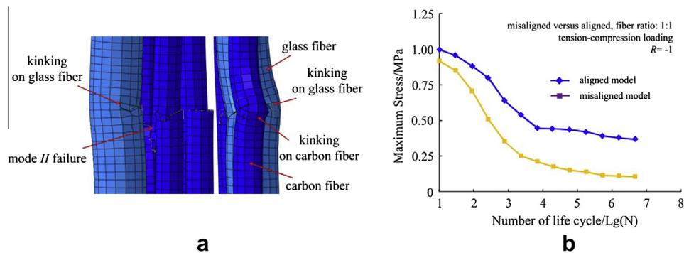
Fig. 16. Observed damage mechanisms in a misaligned hybrid composite under T-C loading (a) and *S-N* curves (vertical axis is normalized by 256.36 MPa).
