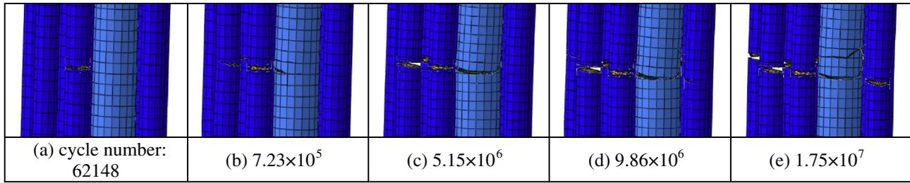
Fig. 3. Crack evolution in a hybrid composite (with carbon/glass volume ratio 3:1).
