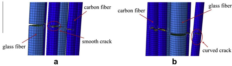
Fig. 9. Crack formation in aligned (a) and misaligned (b) structures.
