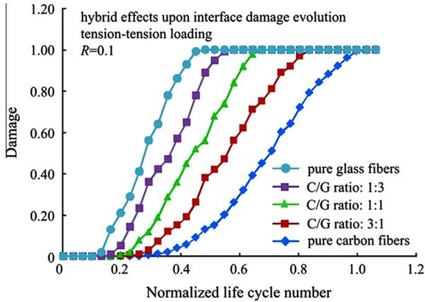
Fig. 6. Interface damage parameter evolution as a function of carbon/glass ratio.
