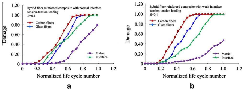
Fig. 4. Damage parameters evolution under tension–tension loading of hybrid FRCs with (a) normal interface (normalized by the cycle number at which the interface is fully damaged,  $2.41 \times 10^6$ ), (b) soft interface (similarly, normalized by  $1.17 \times 10^6$ ).
