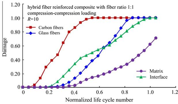
Fig. 13. Damage parameter evolution in 1:1 hybrid composite under compression-compression loading (normalized by the interface lifetime:  $3.74 \times 106$ ).
