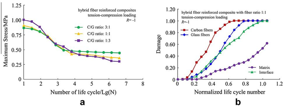
Fig. 14. *S-N* curve and damage parameter evolution of hybrid FRC under T-C loading (a) *S-N* curves, (b) damage parameter evolution in 1:1 hybrid FRC. Vertical axis is normalized by 302.21 MPa.
