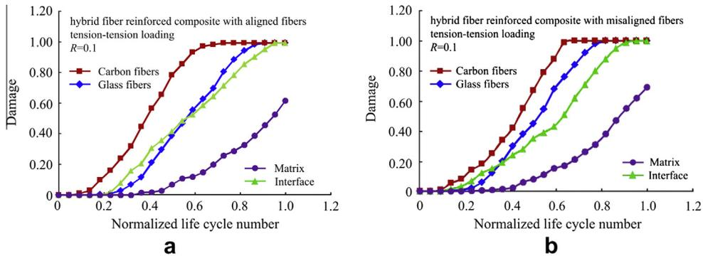
Fig. 10. Damage parameter in main phases plotted versus the life cycle number (a) composite with aligned fibers (normalized by the interface lifetime of  $4.16 \times 10^6$ ) (b) composite with misaligned fibers (normalized by the interface lifetime of  $3.12 \times 10^6$ ).
