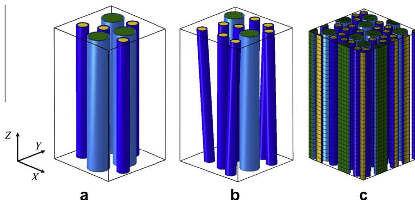
Fig. 1. 3D unit cell models of hybrid composites (a) unidirectional (carbon/glass volume ratio: 1:3), (b) misaligned (carbon/glass volume ratio: 1:1), (c) multi-fiber FE model with fibers cut by the borders.
