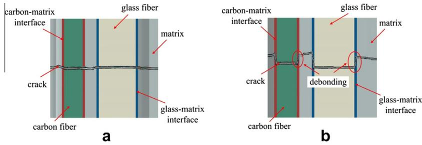
Fig. 5. Micromechanisms of the interface properties effect of hybrid composites (a) normal interface, (b) soft interface.
