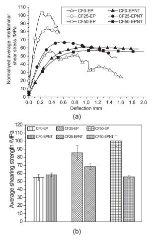
**Fig. 4.** Normalized interlaminar shear stress-deflection curve (a) and average interlaminar shear strength (balk diagram) (b).
