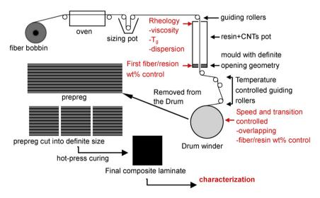
Fig. 2. Schematic view of composite preparation.
