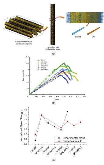
Fig. 7. Multiscale finite element model of the composite with 50% CNTs in sizing (a) and simulated stress-strain curves (b) and model-experiment comparison (c).
