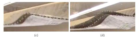
Figure C.19: (a) Sequence of the trailing edge failure just before trailing edge separation, (b) in the beginning of the trailing edge separation, (c) at the opening sequence of the trailing edge failure and (d) subsequently sequence with increased separation.
