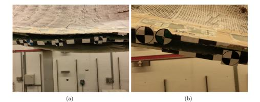
Figure C.20: Trailing edge opening after blade failure. (a) Trailing edge separation from the bondline and (b) cracked bondline.
