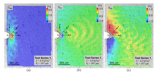
**Fig. 15.** The contour plots of  $\varepsilon_{\theta\theta}$  (a),  $\varepsilon_{rr}$  (b), and  $\varepsilon_{\theta r}$  (c) captured at magnification ×100.
