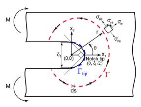
Fig. 2. Contours used for the J-integral determination.
