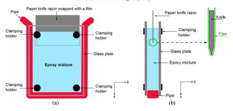
**Fig. 4.** Manufacturing of specimens in *x-z* plane (a) and *x-y* plane (b).
