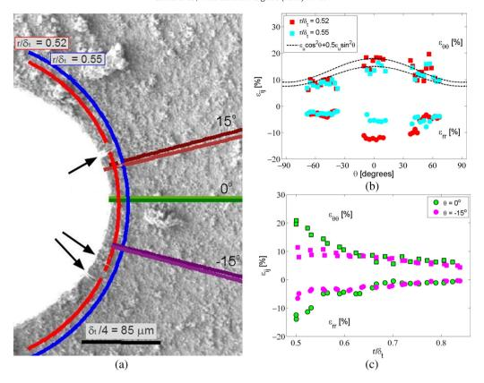
Fig. 8. The notch loaded with  $J=11.7 \text{ k}/\text{m}^2$  and the corresponding strains along circumferential and radial paths (a). Micro-cracks are indicated by arrows. The associated strain components  $ε_{\theta\theta}$  (squares) and  $ε_{rr}$  (circles) are shown as a function of circumferential position (b) and as a function of radial position (c).
