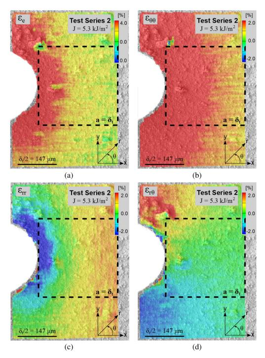
Fig. 13. The strain contour plots for the Test Series 2 at  $J = 5.3 \text{ kJ/m}^2$  (boxes indicate the comparable length scale with the Test Series 1, see Fig. 12; the point of origin is out of view).
