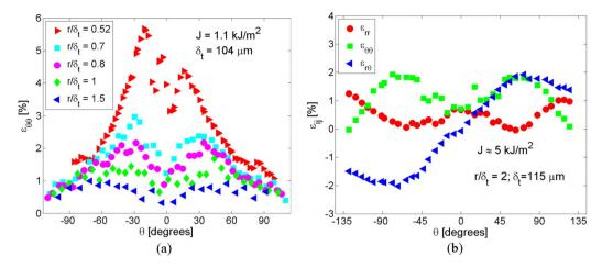
**Fig. 16.** The strain component  $\varepsilon_{\theta\theta}$  is shown as a function of angle around the notch for various distances  $r/\delta_t$  from the notch tip (a); the variations of all strain components with an angle around the notch at  $r/\delta_t = 2$  (b) (results for the Test Series 1).
