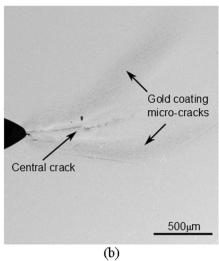
Fig. 18. The damaged surface around the notch without speckles for the Test Series 1 in the unloaded state after applied  $J = 7.2 \text{ kJ/m}^2$  at magnification  $\times 1000$  (a) and  $\times 100$  (b).
