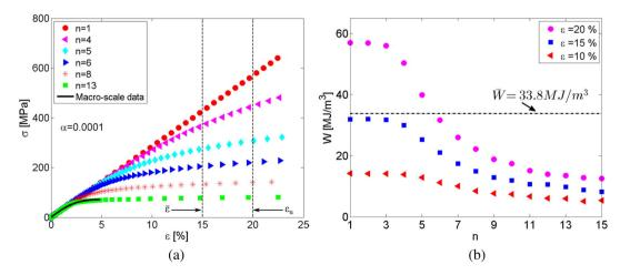
Fig. 9. The stress-strain relations with n within the range of 1–13 for  $\alpha = 0.0001$  (a), and the strain energy density as a function of n for strain limits of 10%, 15%, and 20% (b).
