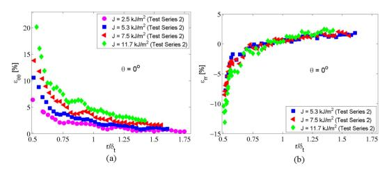
**Fig. 17.** The strains along the line paths at  $\theta = 0^{\circ}$  for  $\varepsilon_{\theta\theta}$  (a) and  $\varepsilon_{rr}$  (b).
