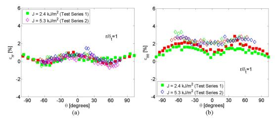
Fig. 14. The strain components  $\varepsilon_{rr}$  (a) and  $\varepsilon_{\theta\theta}$  (b) are the angle as a function of angle around the notch at  $r/\delta_t = 1$  (Load Set 2). Filled markers correspond to the Test Series 1 and open markers to the Test Series 2. Different colours indicate different specimens within test series. (For interpretation of the references to color in this figure legend, the reader is referred to the web version of this article.)
