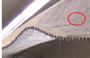
Figure 8: Trailing edge deformation just before reaching the ultimate load (right). Note the distinct kink at the upper surface.
